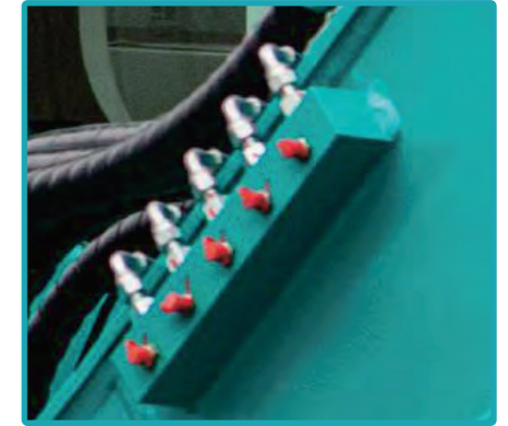
Centralized lubrication of boom and one-stop application of grease.
